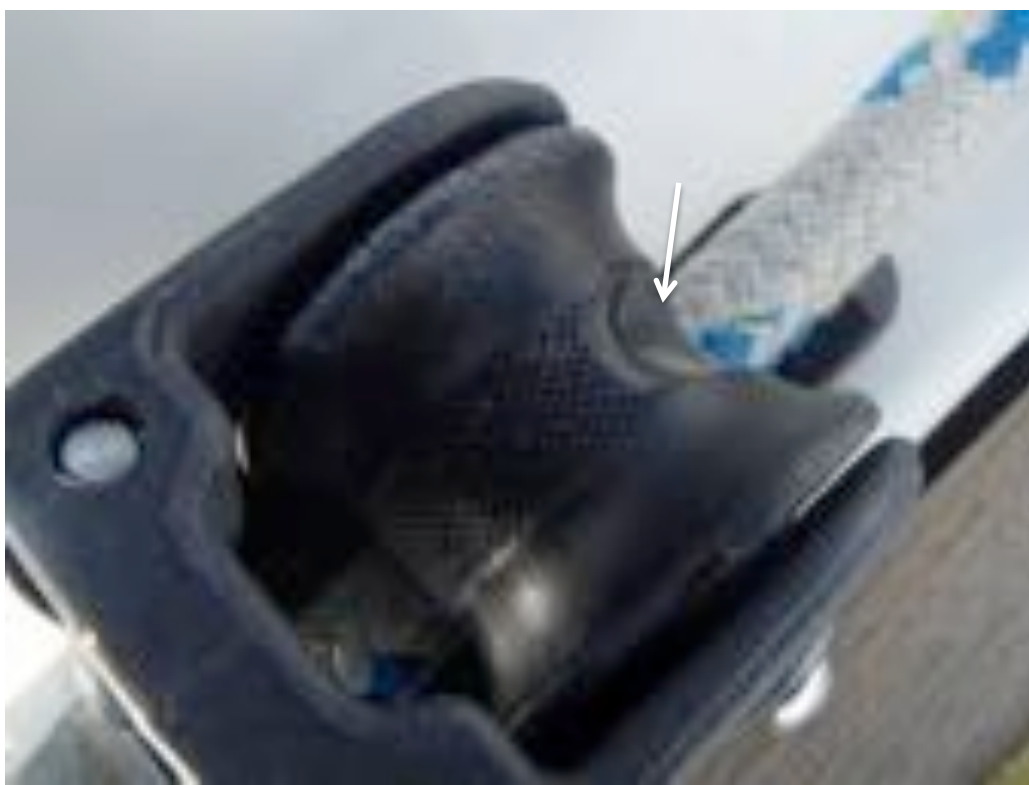
Image of the port side genoa turning block. Note the wear to the sheave.
