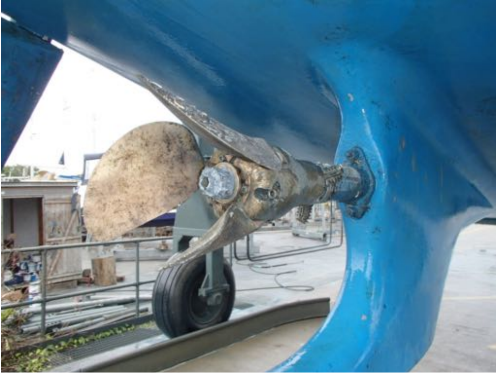
Image of the stern gear. Note the wasted propeller anode
