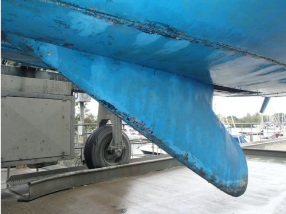
Image of the swing keel partially lowered. Note the surface corrosion developing and absence of antifouling on the leading edge and foot.
