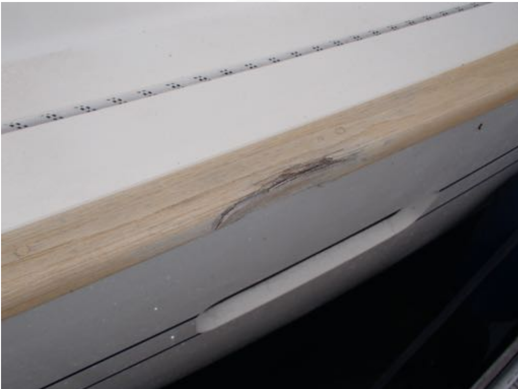
Image of damage noted to the port toe rail
