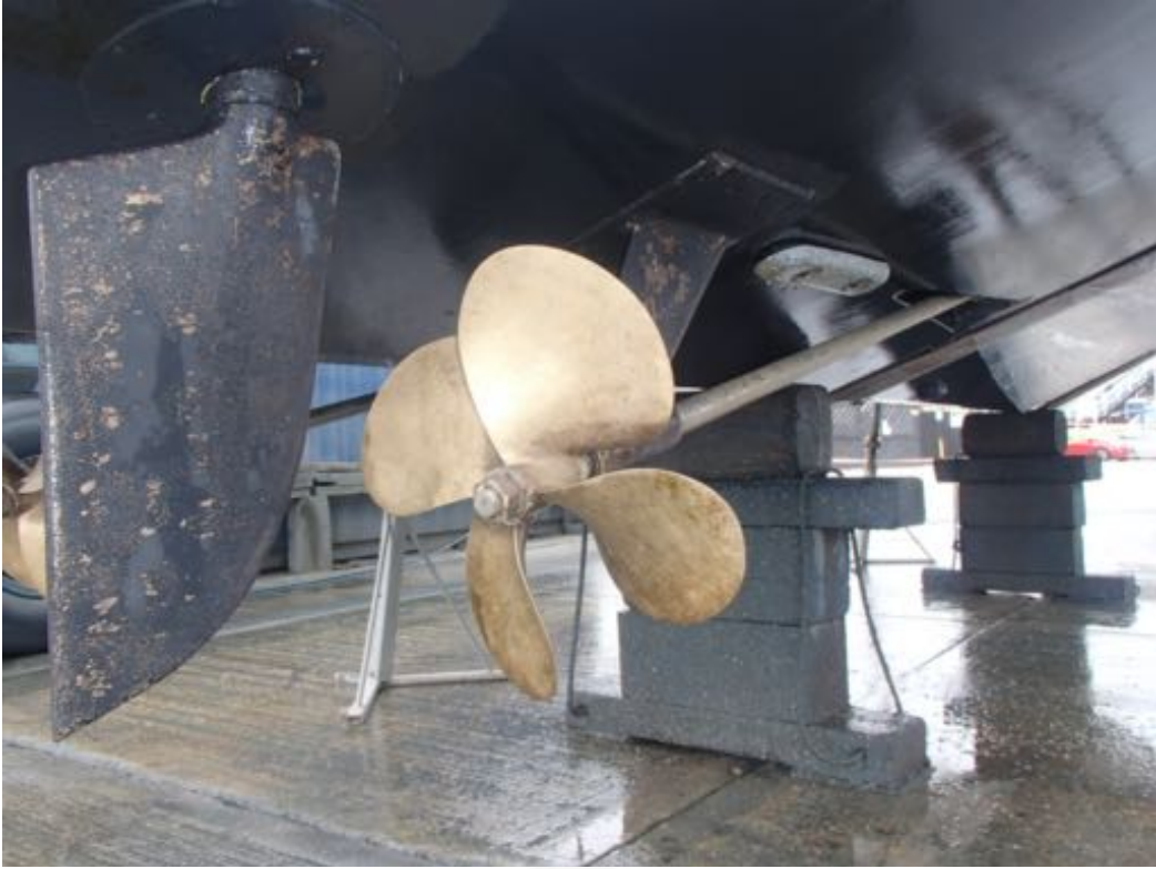
Image of the starboard stern gear post jet wash cleaning.
