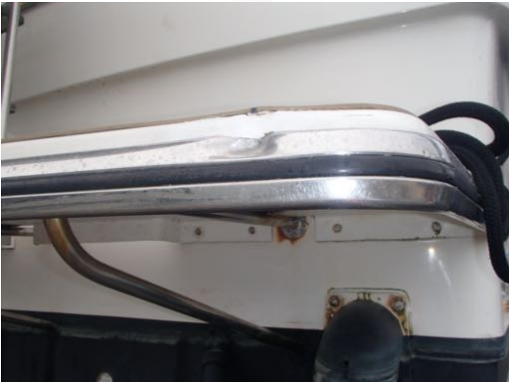
Image of the contact damage to the platform to starboard.
