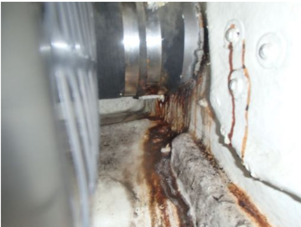
Image of the starboard aft engine exhaust hose weeping where secured to the transom fitting.
