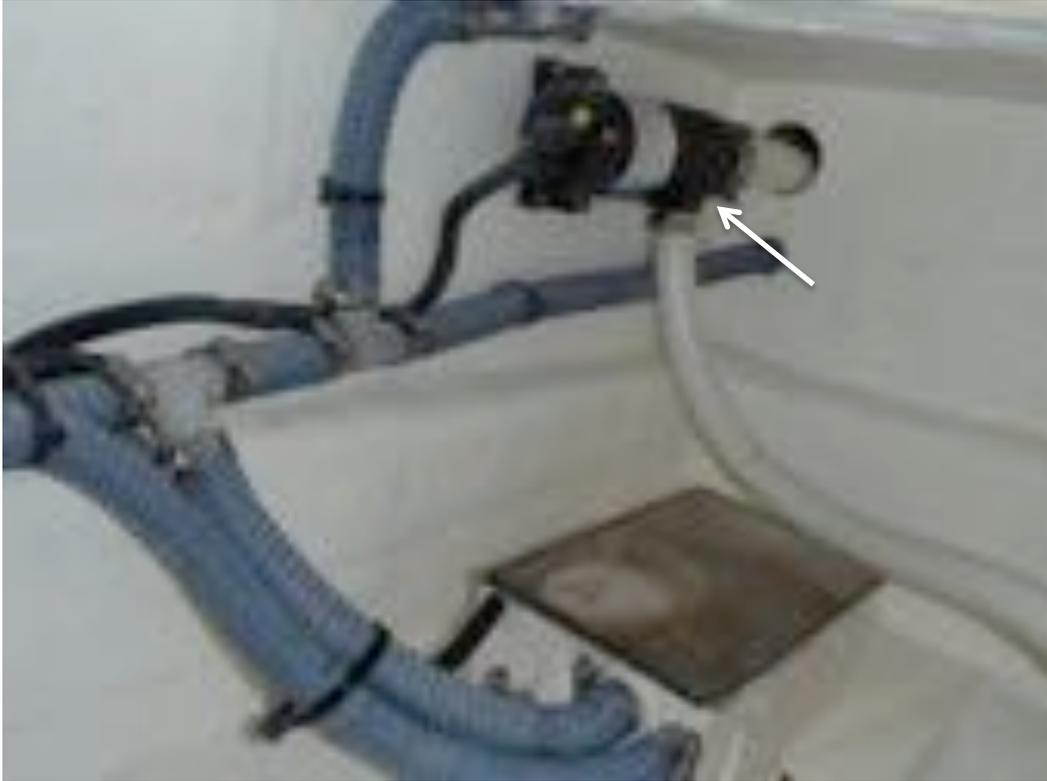
Image of the macerator pump which was found to be defective.
