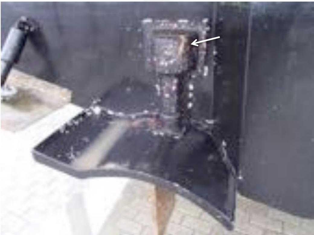
Image of the transom cover. Note evidence of a past repair.
