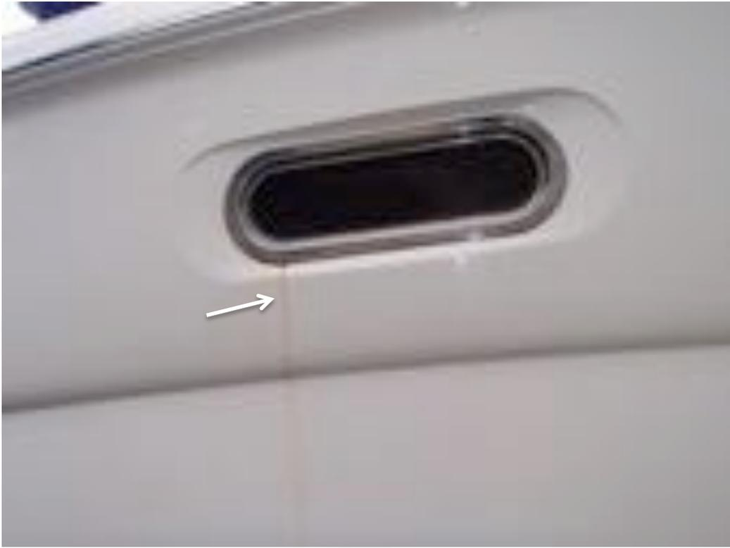
Image of the starboard forward portlight. Note the rust streaking.
