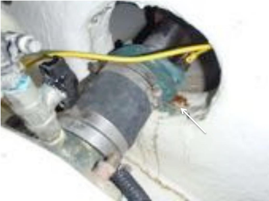
Port shaft seal. Note the surface corrosion developing and weep at the base.
