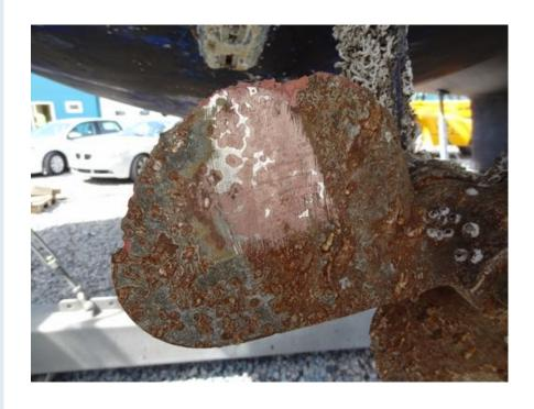
Classic dezincification noted on a propeller. The pink colour is where the Zinc in the alloy has been removed due to corrosion leaving a Copper rich alloy. A Copper rich alloy is brittle and weak. When this propeller was struck with a hammer it shattered like glass!
