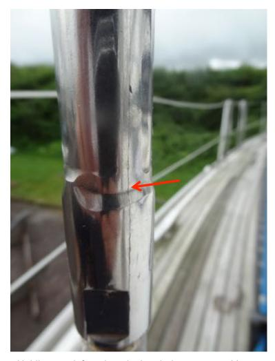
Hairline crack found on rigging during a survey. Very faint and difficult to see, but significant.
