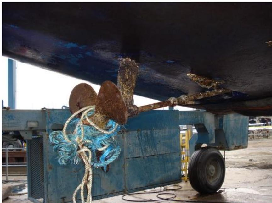
Fouling noted on the stern gear of a vessel lifted for a survey. Fouling such as this can result in damage to the cutlass bearing, shaft or even the P-Bracket. The use of a rope cutter can reduce the likelihood of fouling such as this.
