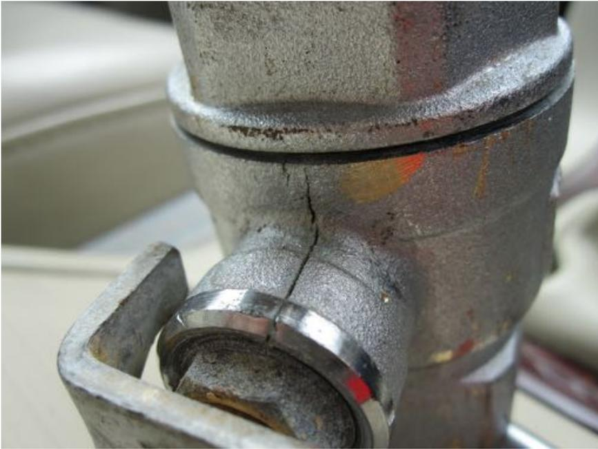
Crack found in the body of a seacock valve.
