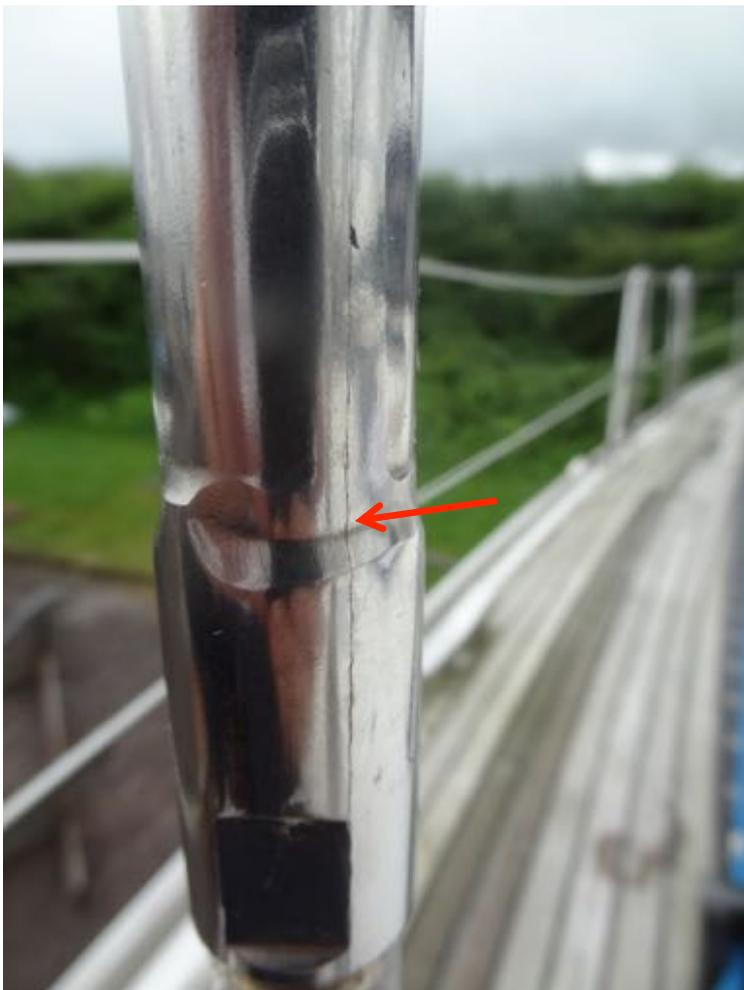
Hairline crack found on rigging during a survey. Very faint and difficult to see, but significant.
