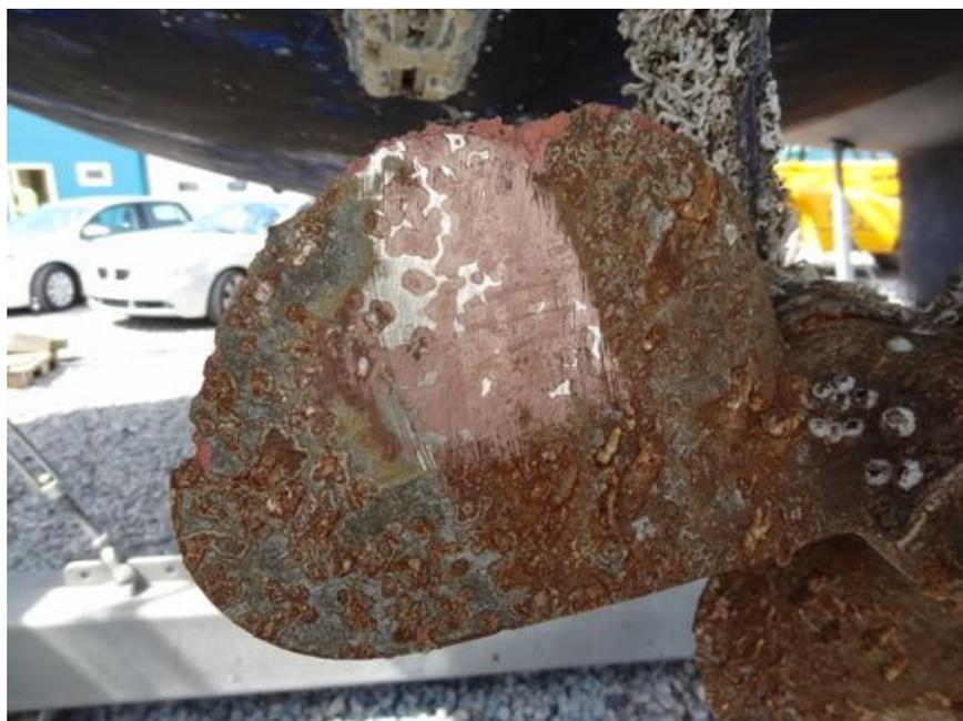
Classic dezincification noted on a propeller. The pink colour is where the Zinc in the alloy has been removed due to corrosion leaving a Copper rich alloy. A Copper rich alloy is brittle and weak. When this propeller was struck with a hammer it shattered like glass!
